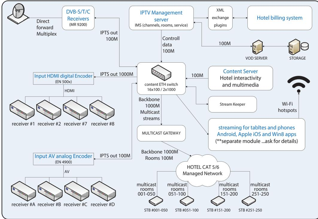
IPTV Operator with centralized Headend/Stream Provider
