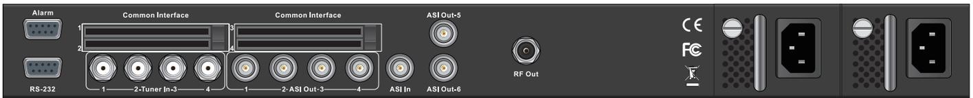
Back Panel GX 5204/8 Multireceiver + Encoder / Transmodulator
